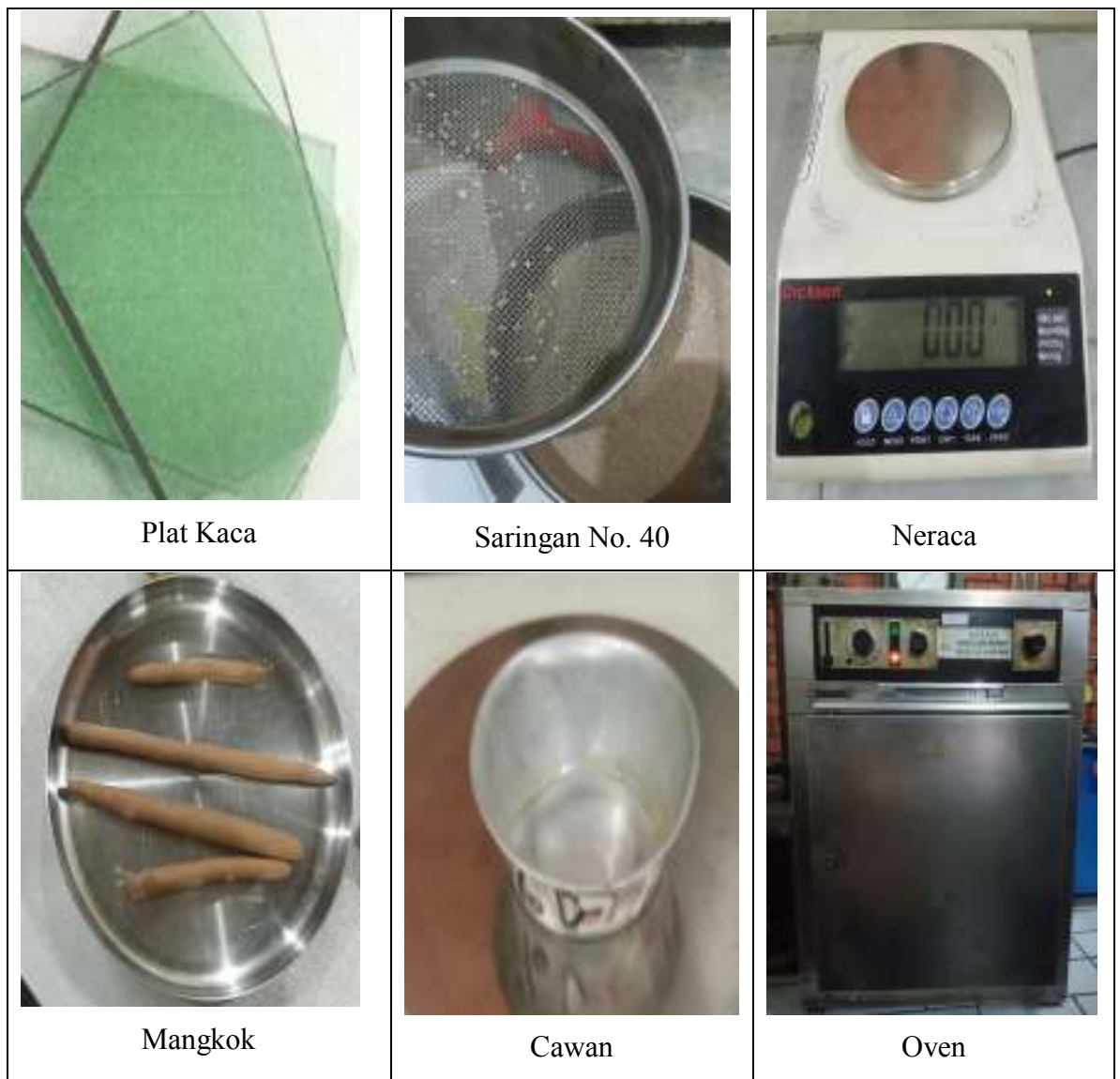
Gambar 3.7 Alat Percobaan Analisa Batas Plastis ( Plastic Limit )
