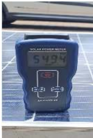
Gambar 3. 3 Solar Power Meter
