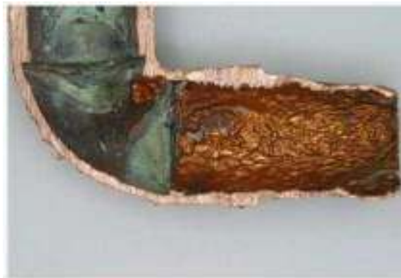
Gambar 2. 10 Korosi erosi (Sumber : Jaya, dkk, 2010)
