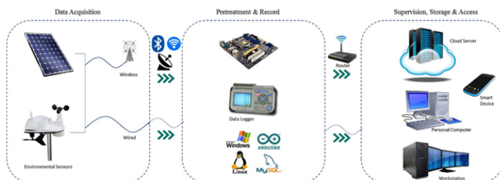
Gambar 5.2.: Arsitektur Sistem Monitoring Panel Surya (Kamenopoulos and Tsoutsos, 2015)
