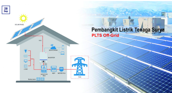
Gambar 10.3: Sistem PLTS Off-Grid
