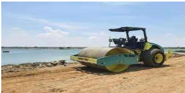
Gambar 2.5 Alat Berat Vibratory Roller (Sumber : Diah Lydianingtias, 2018)
