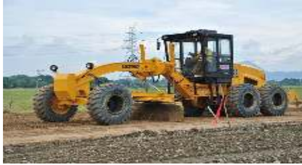
Gambar 2.6 Alat Berat Motor Grader (Sumber : Diah Lydianingtias, 2018)
