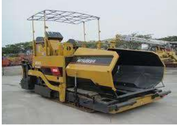
Gambar 2.9 Alat Berat Asphalt finisher (Sumber : Diah Lydianingtias, 2018)
