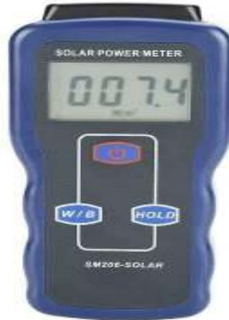
**Gambar 3.1 Solari Meter**
