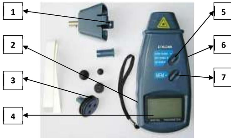
**Gambar 3.4 Tachometer Digital**
