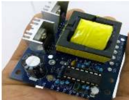
Gambar 3. 5 Modul Inverter 150W 12V DC to AC
