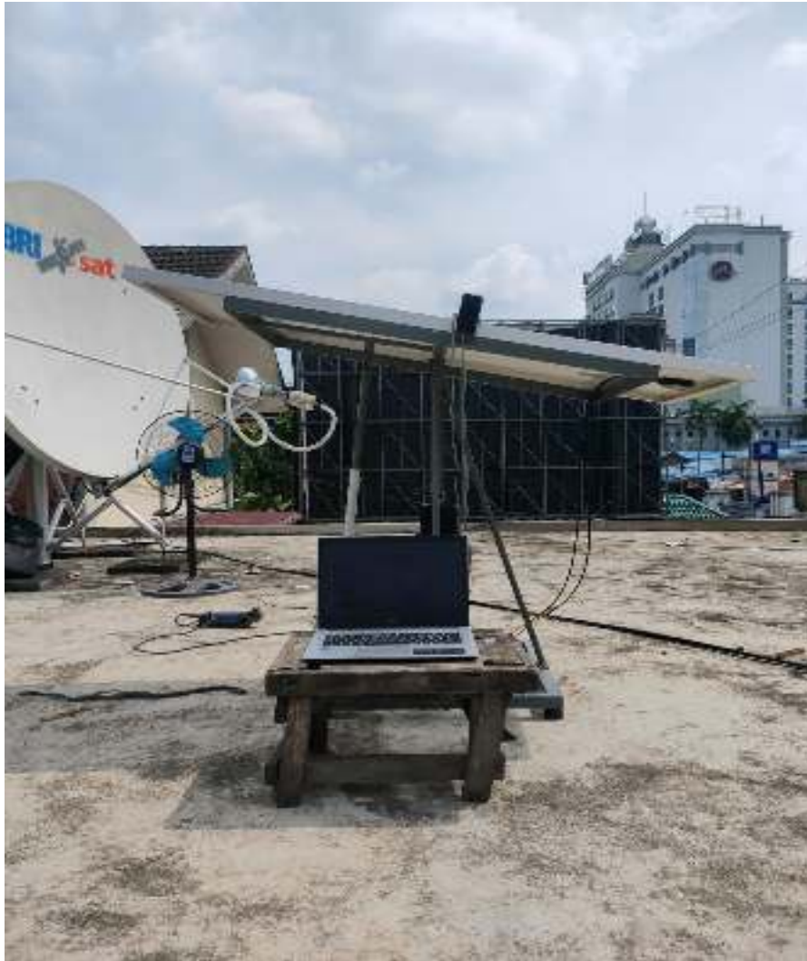
Gambar 3.23: Gambar Single Axis 5 ° solar tracker (utara selatan)
