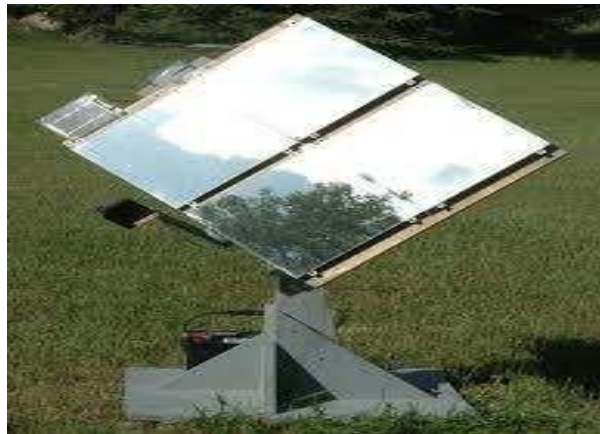
Gambar 2.23. Multi-mirror Reflective Unit
