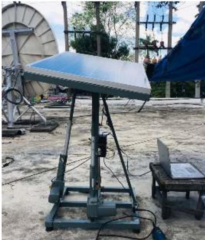
Gambar 3.22 : Gambar *Double Axis solar tracker*
