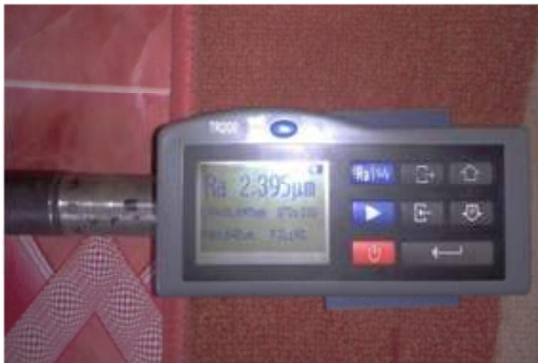
**Gambar 2.16** *sureface roughness tester type TR200*
