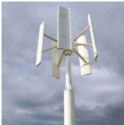
Gambar 2.11 Blade wind turbine Sumbu Vertikal
