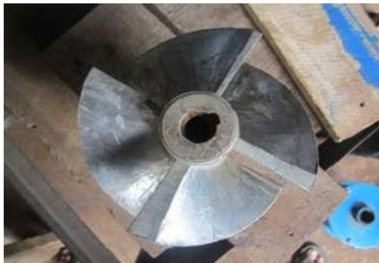
Gambar 2.9. Turbin Propeller
