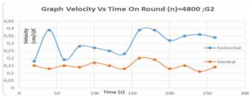
Graph 3.5 Speed with time relationship at n = 4800 rpm, G2
