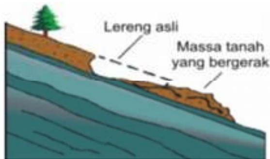
Gambar 2.5 Aliran/*Flow*
