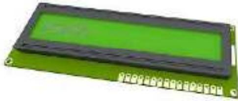
Gambar 2.17: *Liquid Crystal Display (LCD)*
