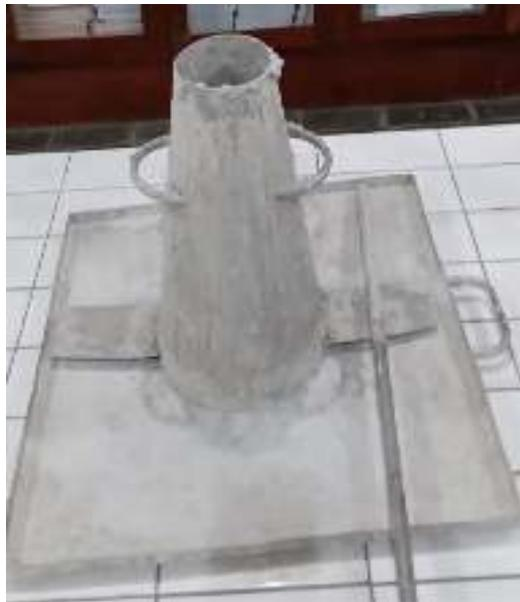
Gambar 2.6 Kerucut Abrams
