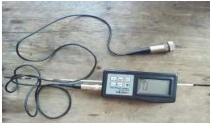
Gambar 3.3 Vibrometer *Handheld*
